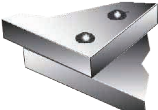
Plug Welds (Fig 1-19j)
